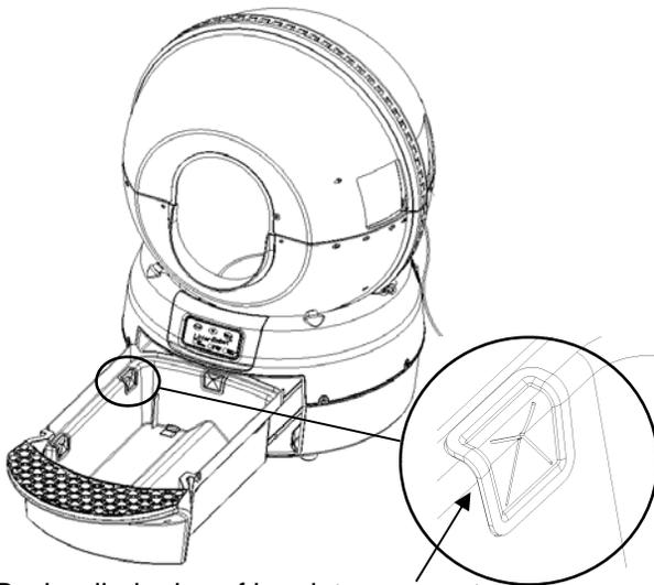
Push rolled edge of bag into grommets
