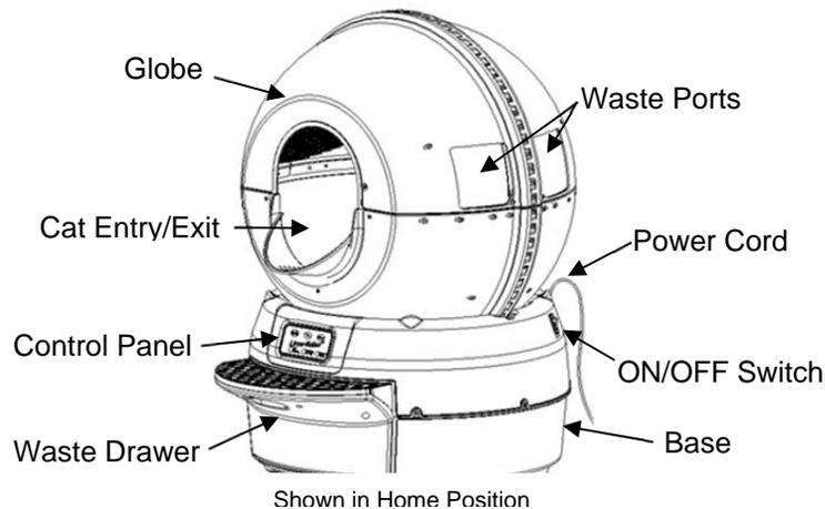
3. Plug the small connector from the AC adapter into the socket in the back of the Base unit. Next, plug the main power cord into a wall outlet. Press the ON/OFF Switch - the Litter-Robot will perform an initialization cycle (this takes about 3 minutes). After completing the cycle, the Globe should be in the "home" position with the green light on.
