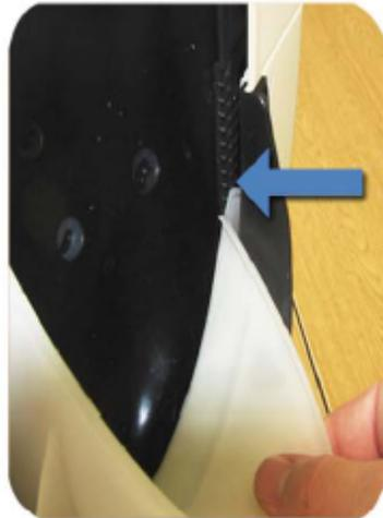
3. Make sure tab is between Guard Lever and Liner.
