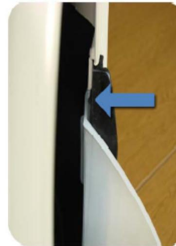
6. Make sure Extender tabs lock in beneath the upper Globe flanges (both sides).
