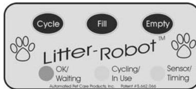
3. If the red light is on ("Sensor/Timing"), push any of the buttons (Cycle, Fill, or Empty). This resets the unit and the green light should come on ("OK/Waiting"). Next, proceed to Step 4 of this Testing procedure.
