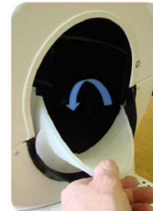
2. Rotate Extender with flange starting to overlap Rubber Lip.
